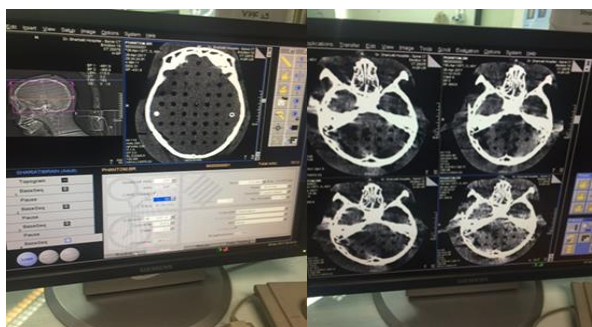
Figure 5. Images from scanning the phantom, assessed by four experienced examiners to evaluate the effect of radiation reduction on the image quality
