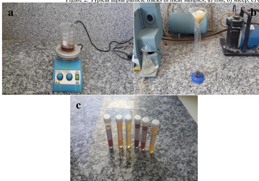
Figure 3. Process of sample preparation; a) heater, b) filtration, c) test tube
