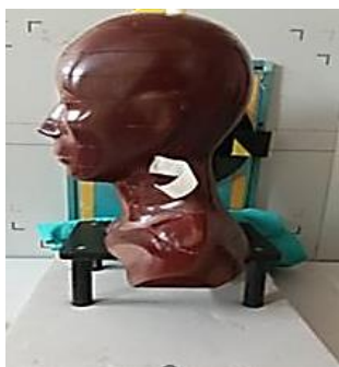
Figure 1. Experimental setup of the phantom for the lateral cervical radiography
