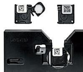
Figure 3. Illustration of a) OSLD nanoDot b) OSLD in situ in the inLight MicroStar Reader
