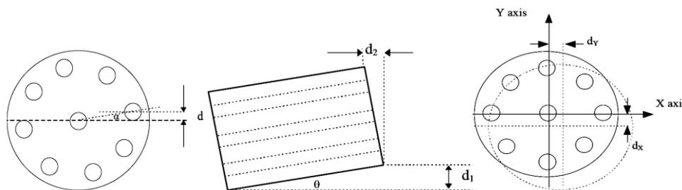
**Figure 3.** From right to left: lateral, angular, and rotational deviations of the phantom in CT scanner
