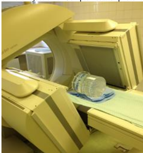
Figure 1. Acquisition of 2D projections of the phantom using a Siemens E-cam dual-head gamma camera
