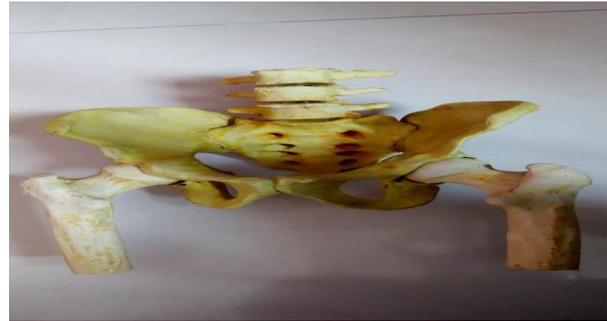
Figure 2. A male pelvis and femur bone used in a developed phantom
