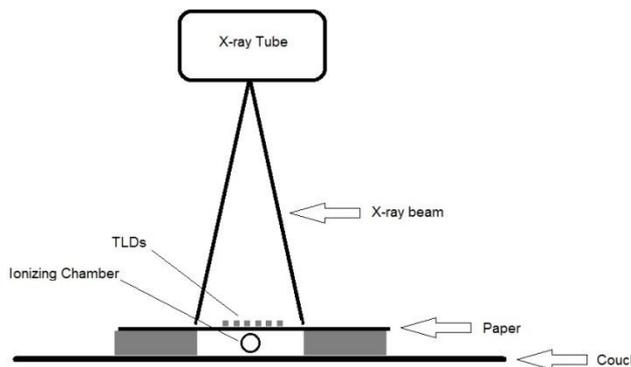
Figure 3. Experimental setup used for TLD calibration
