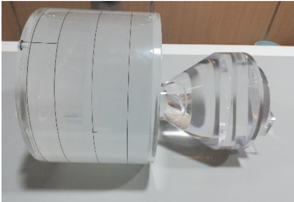
Figure 1. Water (circular) and acrylic (Cone) phantoms in a position of the scanning. The model is scanned by two different CT (Sinovision, Instium 16) protocols (A and B) where (A: 120 KV /150 mA, FBP ; B: 120KV/ (20-150 mAs, IDREAM).
