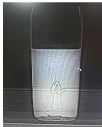
Figure 1. Computer tomography scout image of chicken leg phantom
