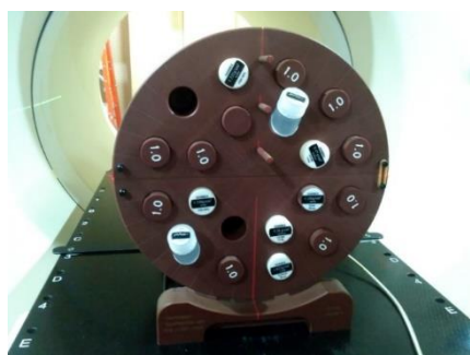
Figure 1. The Cheese phantom with 20 plugs of 10 different densities.
