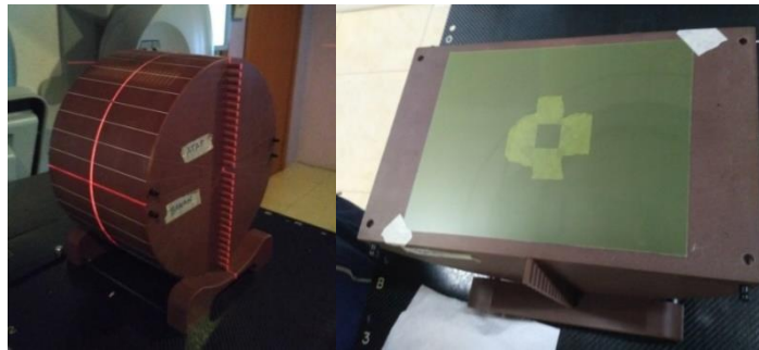
Figure 2. Cheese phantom set up for DQA (left) and Film placement, inserted in the middle of the cheese phantom.
