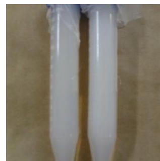
Figure 4. Irradiated tubes (left: 0 Gy, right: 15 Gy)
