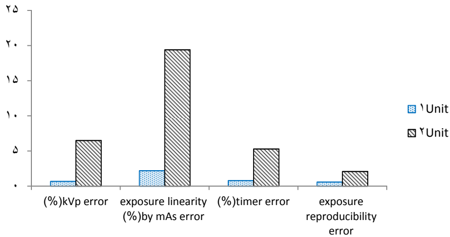
Figure 4. Results related to the accuracy of the output voltage (kVp), linearity of exposure with mAs, timer accuracy, and reproducibility of the exposure in Shahid Hashemi Nejad Hospital.
