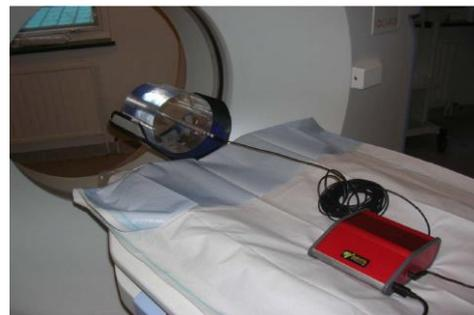
Figure 2. CTDI phantom and pencil dosimeter chamber [8]
