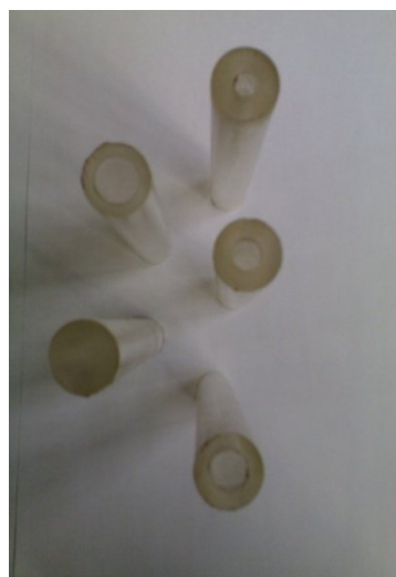
Figure 4. PMMA cylinders with 20 mm diameter
