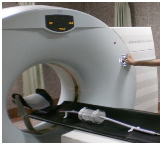
Figure 6. The procedure for the phantom CT scanning.
