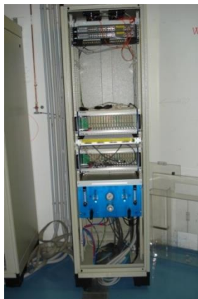
Figure 2. The electronics rack containing a data acquisition system, a power supply, and a gas panel.
