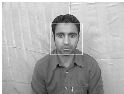
Figure 3. A face detected by Viola-Jones face detector
