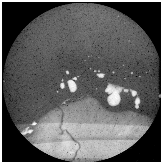
Figure 3. Defects on a newly purchased shield
