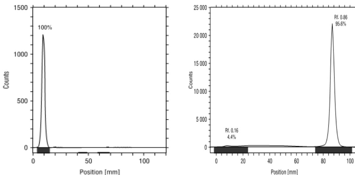
Figure 1. ITLC of  $[^{67}\text{Ga}]\text{GaCl}_3$  (left) and  $[^{67}\text{Ga}]\text{-ATSS}$  (right) on Whatman No. 2 paper, using 10% ammonium acetate:methanol (1:1)
