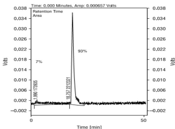
**Figure 2:** HPLC chromatograms of [<sup>67</sup>Ga]AATS solution on a reversed-phase column, using acetonitrile + 0.1% TFA/water + 0.1% TFA, 90:10
