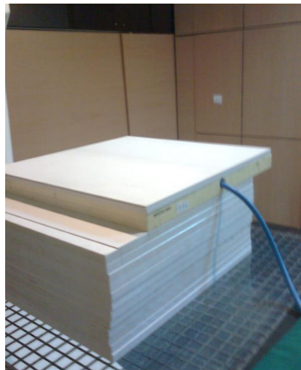
Figure 3. Displacement of the ionization chamber out of the central beam axis by shift by the slab where the
