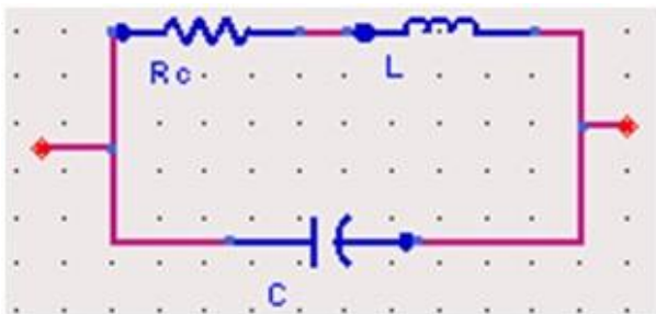
Figure 5. Electrical model of planar microcoil
