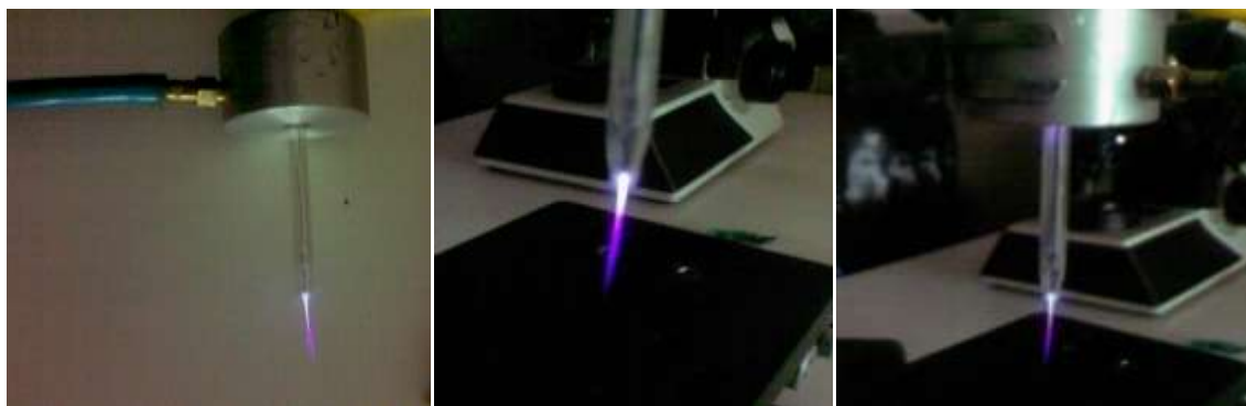
Figure 1. Cold-plasma generating device. Seven cm of the length of the movable electrode is inside the glass tube
