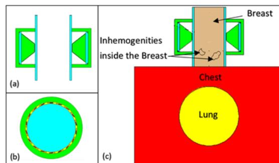
**Figure 1.** a) AccuBoost system, b) Source dwell positions in each applicator, c) Phantom geometry
