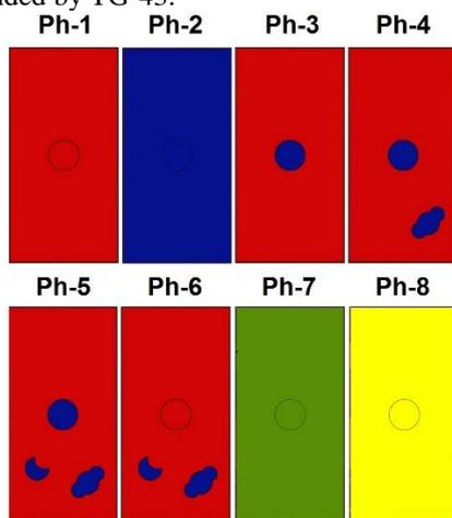
**Figure 2.** Simulation geometry of the breast (mean adipose tissue (red), mean glandular tissue (blue), ICRU-44 breast tissue (green), and normal breast tissue (yellow)) for Ph-1 to Ph-8 phantoms.
