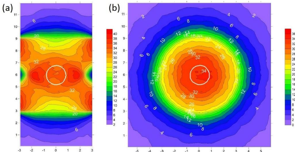
Figure 3. The isodose plots inside the water phantom for the radiation of AccuBoost device (Gy) in a) X-Z direction and b) Y-Z direction
