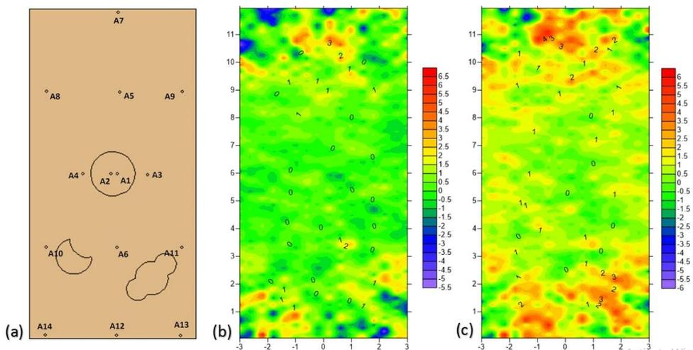
Figure 4. (a) Selected dosimetric point locations; differences obtained from Equation 1 into the breast in X-Z direction for (b) ph-5; and (c) ph-7 phantoms.
