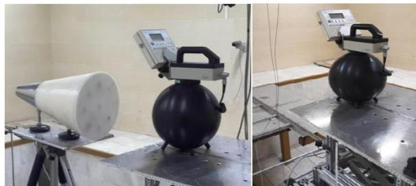
**Figure 2.** Experimental setup for measuring the direct and scattered components of ambient dose equivalent  $H^*(10)$  using Berthold LB 6411 detector. The left and right setups are corresponding to the scatter and total neutron dose measurements, respectively.
