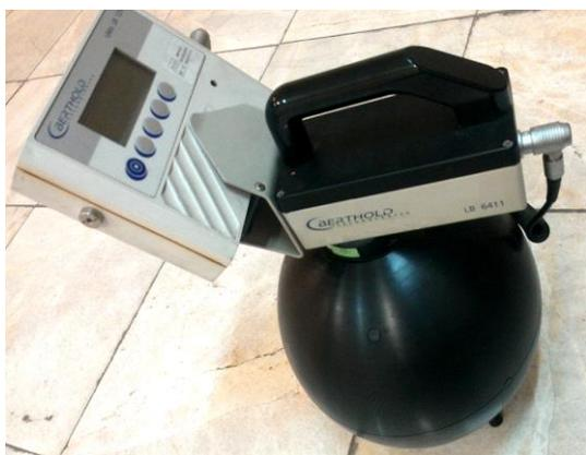
**Figure 1.** Employed Berthold LB 6411 neutron detector in current study
