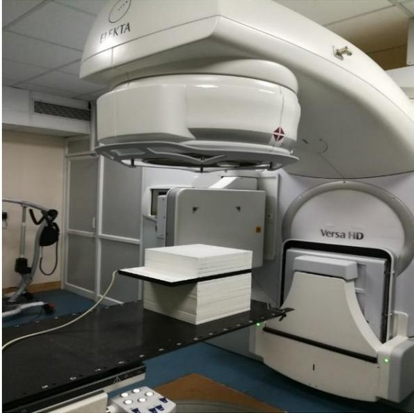
Figure 1. Experimental setup for motorized wedge profile/angle measurement
