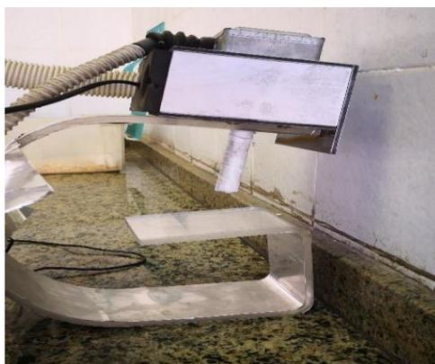
Figure 2. A microwave antenna
