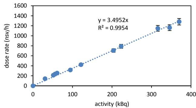
Figure 6. The calibration curve for a detector-to-neck distance of d=11 cm.
