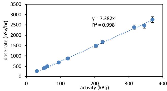
Figure 5. The calibration curve for a detector-to-neck distance of 6 cm.
