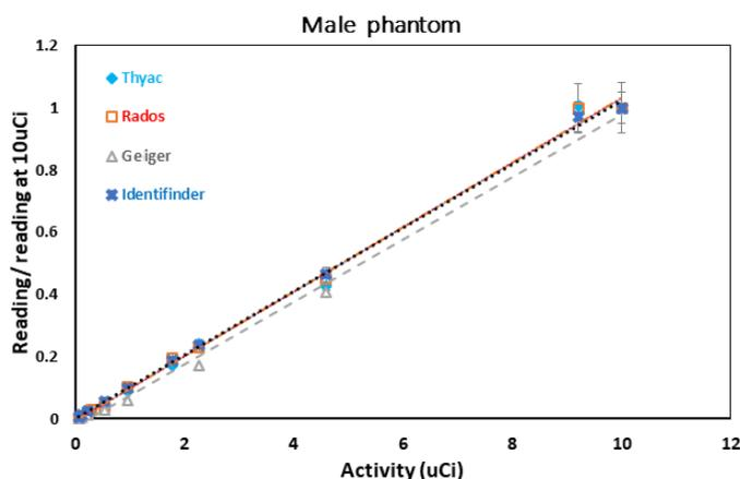
Figure 8. Comparison of calibration curves for the male phantom obtained for different detectors at d=0 cm.
