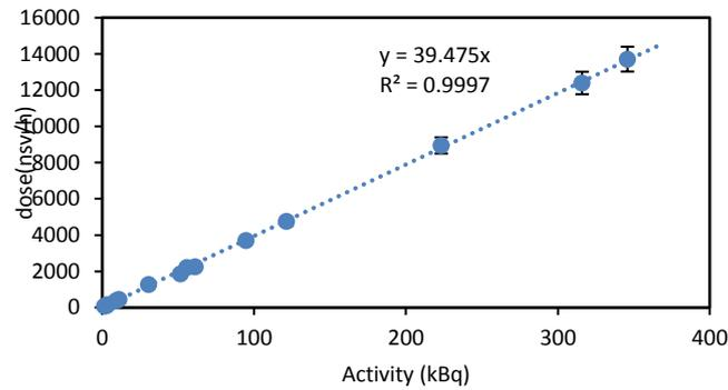
Figure 4. The calibration curve for a detector-to-neck distance of d=0 cm.
