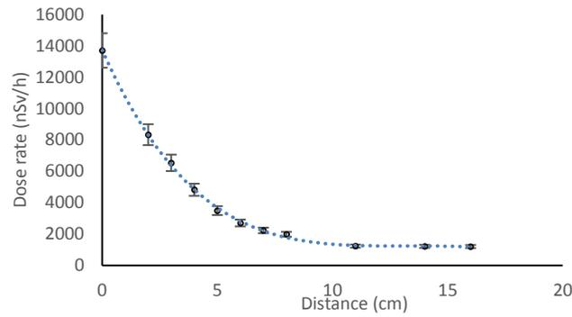
Figure 3: Variations in dose rates at different distances from the thyroid.
