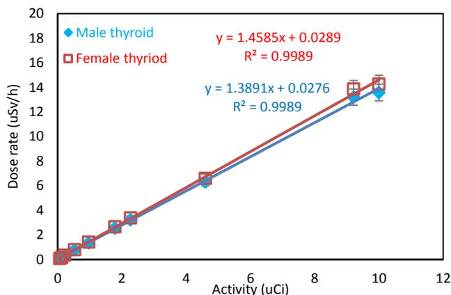
Figure 7. Comparison of calibration curves obtained by the identiFINDER detector for male and female phantoms at d=0 cm.
