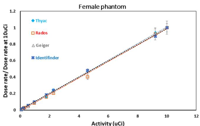
Figure 9. Comparison of calibration curves for the female phantom obtained for different detectors at d=0 cm.
