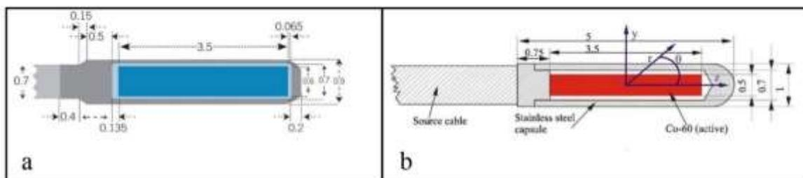
Figure 1. Sources geometries. Dimensions are in mm. (a) Iridium-192 source model mHDR-v2r and (b) BEBIG Cobalt-60 source model Co0.A86 [20,21]
