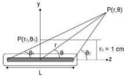
Figure 2. Coordinate system for brachytherapy dosimetry calculations [19].
