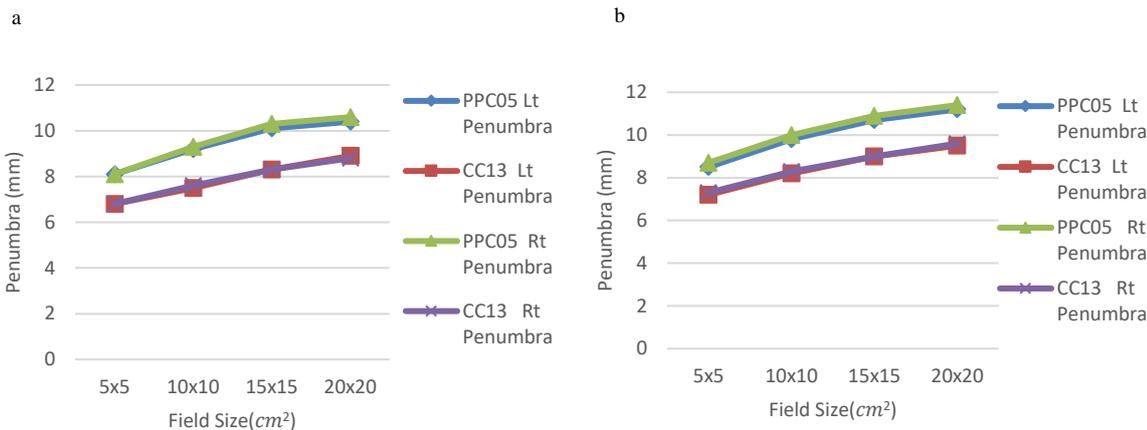
Figure 3. The penumbra width inline (a) and crossline (b) of 6 MV at D<sub>10</sub> for the parallel plate PPC05 chamber and the thimble ionization chamber CC13 at different field sizes.
