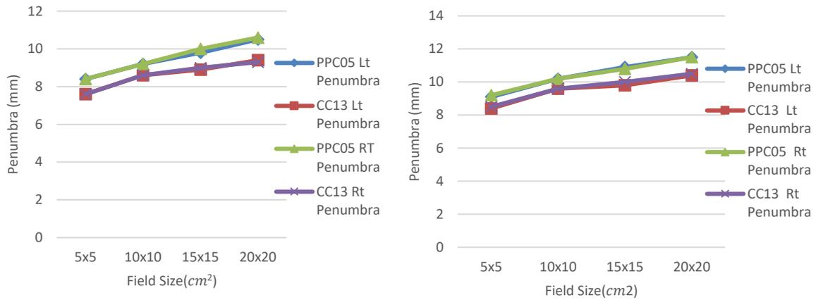
Figure 4. The penumbra width inline (a) and crossline (b) of 10 MV at  $D_{10}$  for the parallel plate PPC05 ionization and the thimble ionization chamber CC13 at different field sizes.
