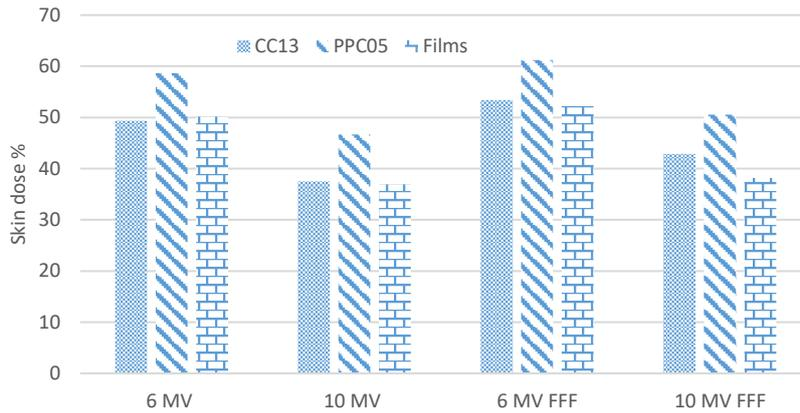
Figure 2. The skin dose of different energies with the parallel plate PPC05 ionization chamber, the thimble ionization chamber CC13, and Gaffchromic films at 10x10 cm<sup>2</sup> field size.
