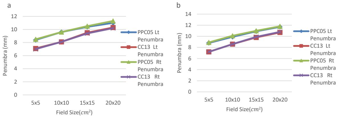
Figure 5. The penumbra width inline (a) and crossline (b) of 6 MV FFF at  $D_{10}$  for the parallel plate PPC05 ionization and the thimble ionization chamber CC13 at different field sizes.
