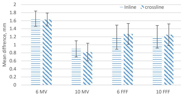
Figure 7. Mean differences of the measurements performed using PPC05 and CC13 chambers for the penumbra regions in inline and crossline dataset at 6 MV and 10 MV with and without flattening filter. Error bars represents 1 standard deviation.
