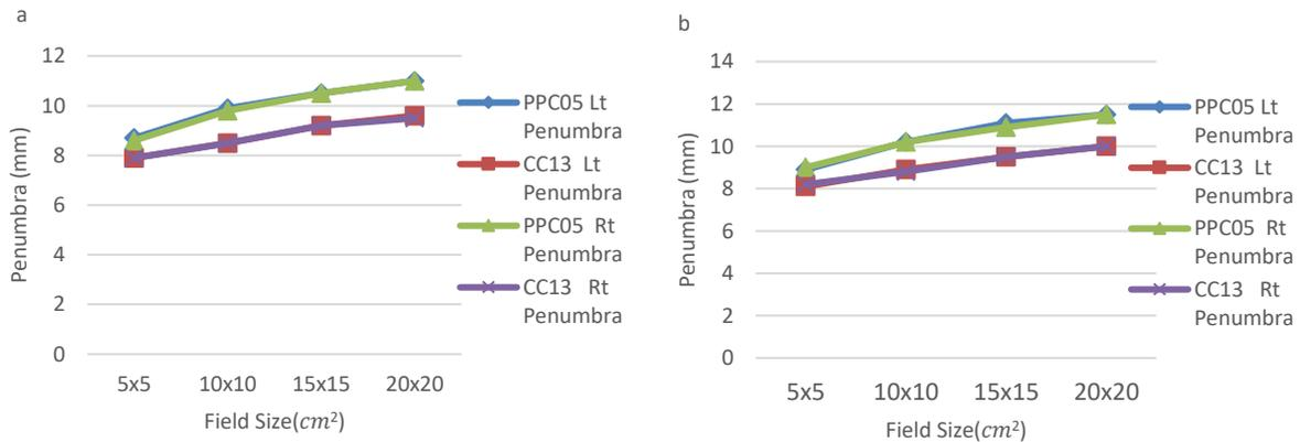
Figure 6. The penumbra width inline (a) and crossline (b) of 10 MV FFF at  $D_{10}$  for the parallel plate PPC05 ionization and the thimble ionization chamber CC13 at different field sizes.
