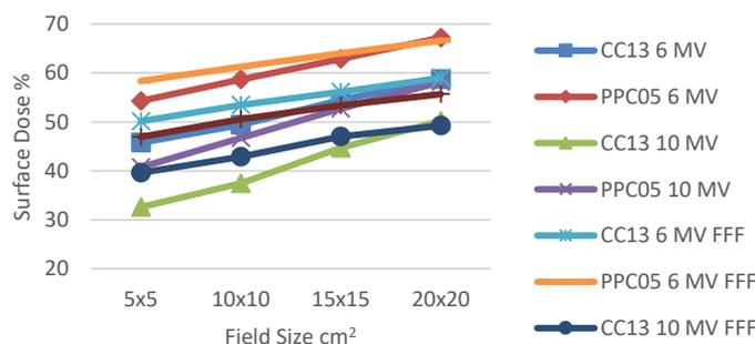
Figure 1. The surface dose with (%) of different energies for the parallel plate PPC05 ionization and the thimble ionization chamber CC13 at different field sizes ( $\text{cm}^2$ ).
