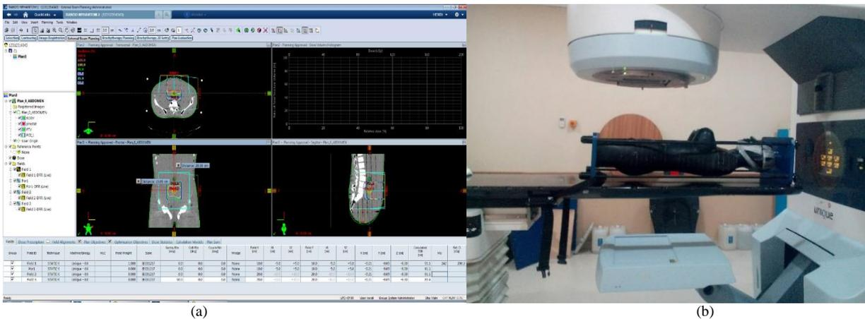
Figure 4. Example of (a) planning on TPS in inhomogeneous phantom; (b) set up Rando phantom and EPID
