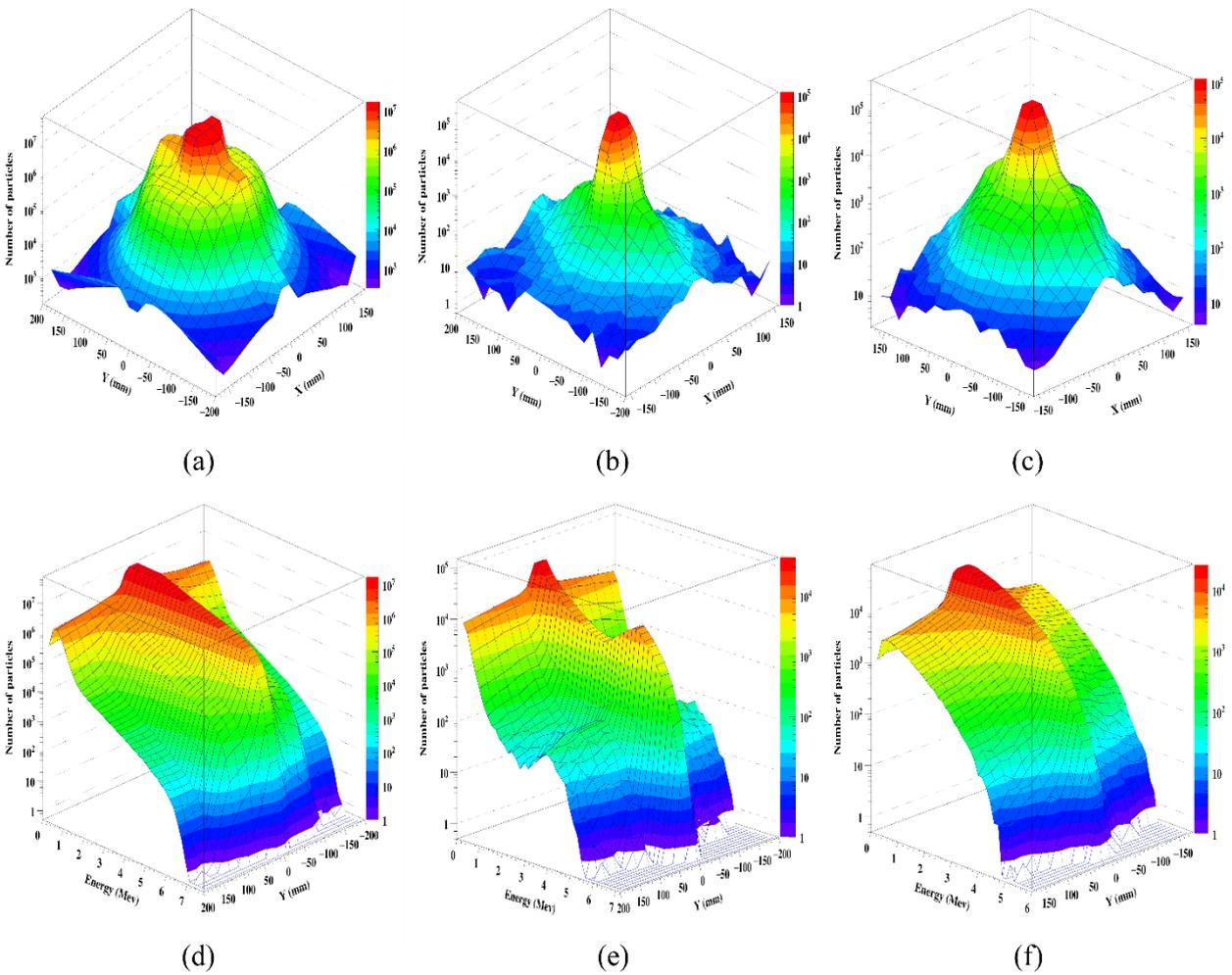
Figure 6. (a) spatial and kinetic energy distribution of leakage and transmitted photons (X-ray) (a, d), electrons (b, e) and positrons (c, f).
