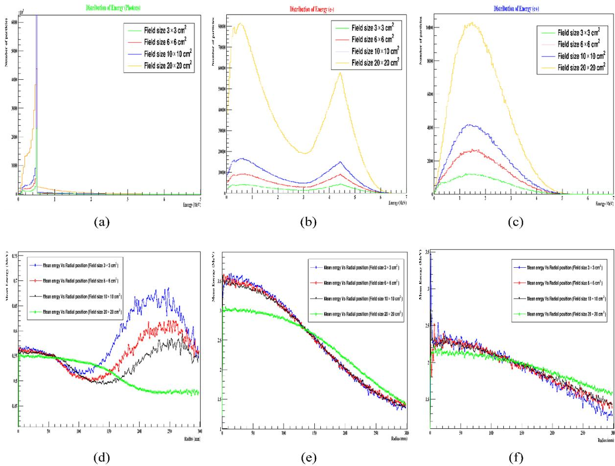
Figure 7. Energy spectra and the mean energy distribution in function of radius of scattered particles for Elekta Synergy 6 MV beams. Photons; (a, d); electrons; (b, e); positrons (c, f).
