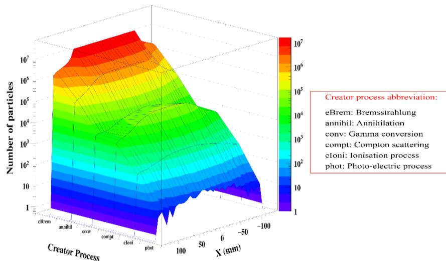
Figure 4. Creator process of particles (Photons, electrons, and positrons) versus the position X(mm) in the surface of Python phase space.
