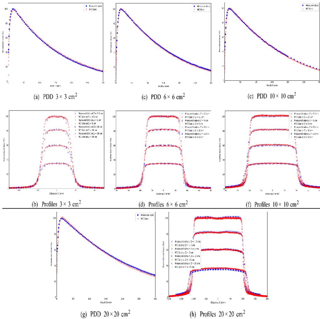
Figure 2. Comparison of simulated and measured PDD's and cross profiles for field sizes ranging from  $3 \times 3$  to  $20 \times 20$  cm<sup>2</sup> for Elekta Synergy MLCi2 linac.
