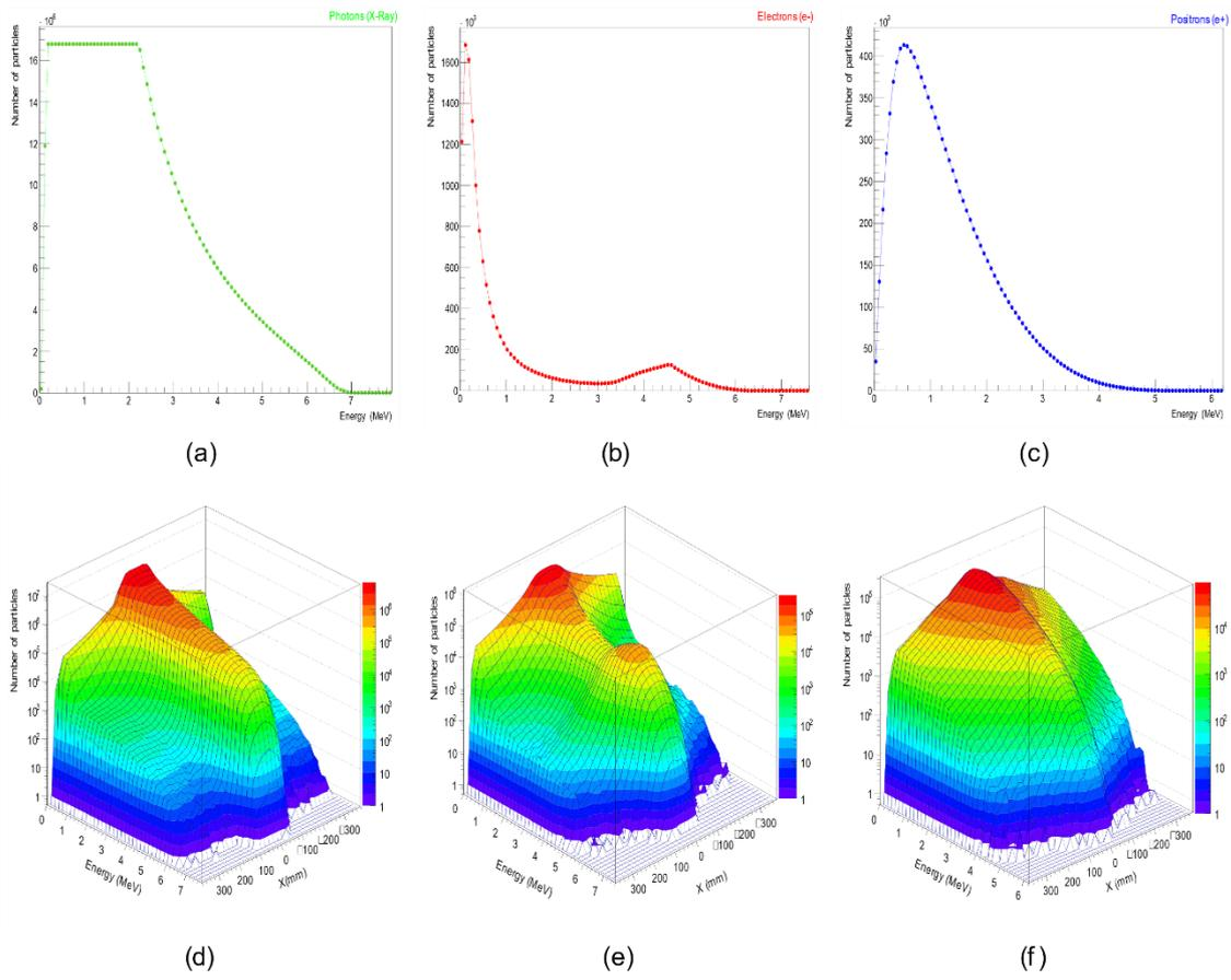
Figure 3. Correlation between coordinates of Python Phase Space. (a, b, c) represents the distribution of the energy spectrum of photons, e- and e+. (d, e, f) exhibits the distribution of X (mm) versus kinetic energy (MeV).
