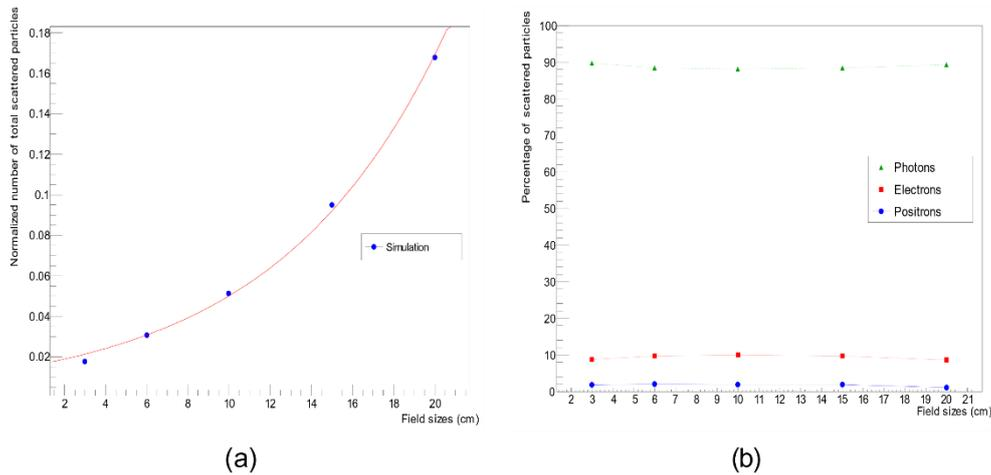
Figure 8. (a) The normalized total percentage of secondary collimator scatter particles in terms of field size for the Elekta Synergy 6 MV MLCi2, fitted using Equation (1). (b) The percentage of scattering photons, electrons, and positrons as a function of field size.
