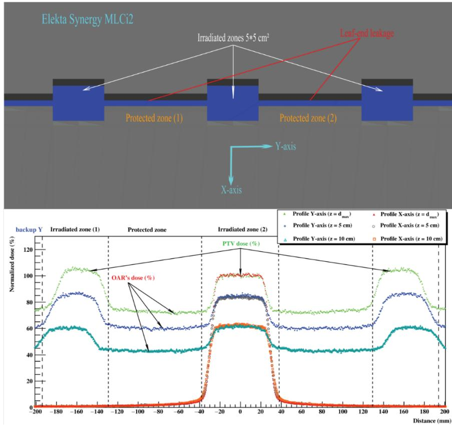
Figure 10. Dose distribution cross profiles in X-axis and Y-axis of a complex plan treatment composed of three sub-fields of size 5x5 cm<sup>2</sup>.
