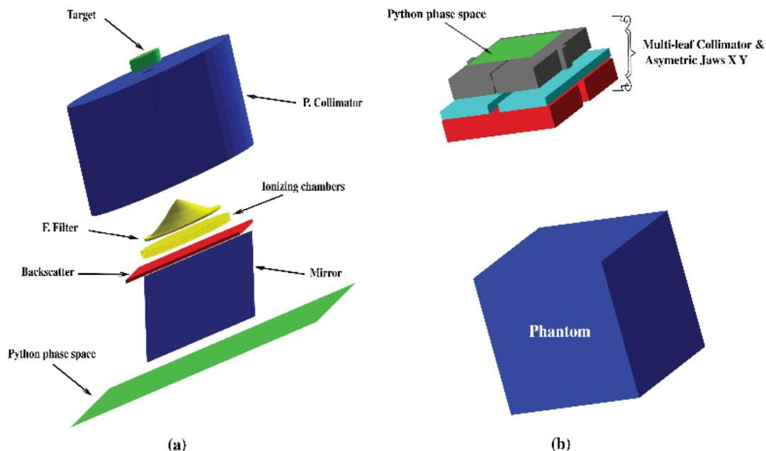
Figure 1. The geometry of the Elekta Synergy MLCi2 system components modeled using the MC Gate 9.0 simulation.
