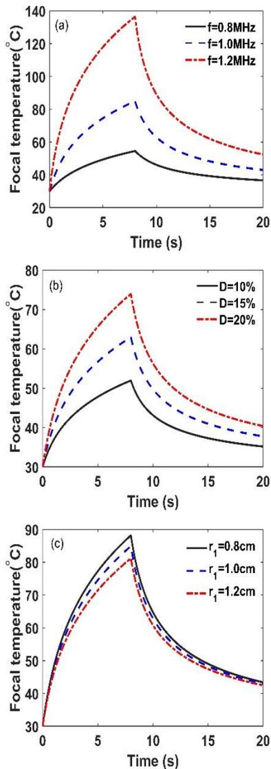
Figure 4. Comparison of focal temperature rise: (a) different frequency; (b) different duty cycle; (c) different inner radius
