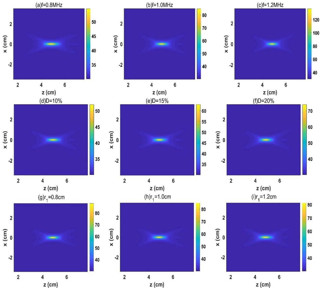
Figure 3. Comparison of temperature contour: a-c different frequency; d-f different duty cycle; g-i different inner radius
