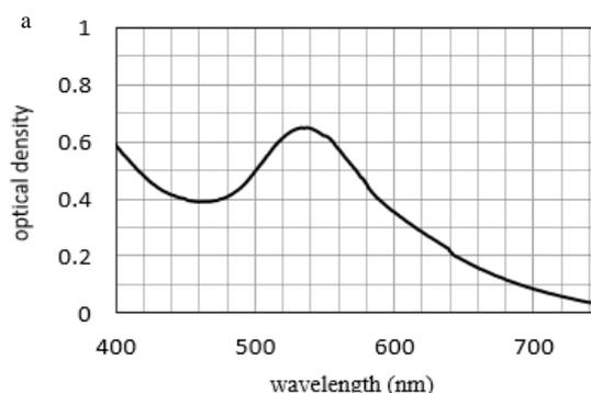
Figure. 1. UV-Vis spectrum of GNPs-Tio Glucose
