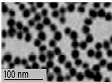
Figure.2. Transmission electron microscopy (TEM) image of the GNPs
