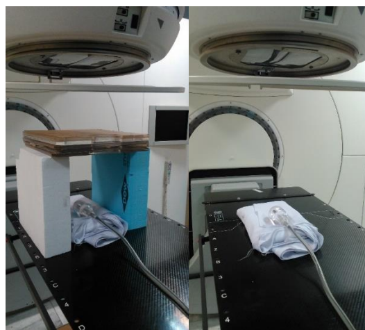
Figure 4. Farmer dosimeter with and without acrylic plates
