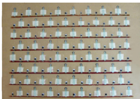
Figure 2. Array of pressure and temperature sensors
