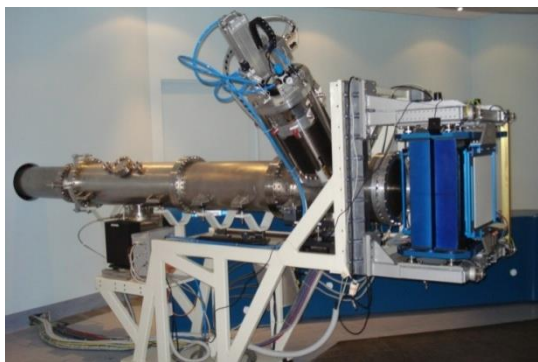
Figure 1. The nozzle with the monitoring system installed in front of the beamline.
