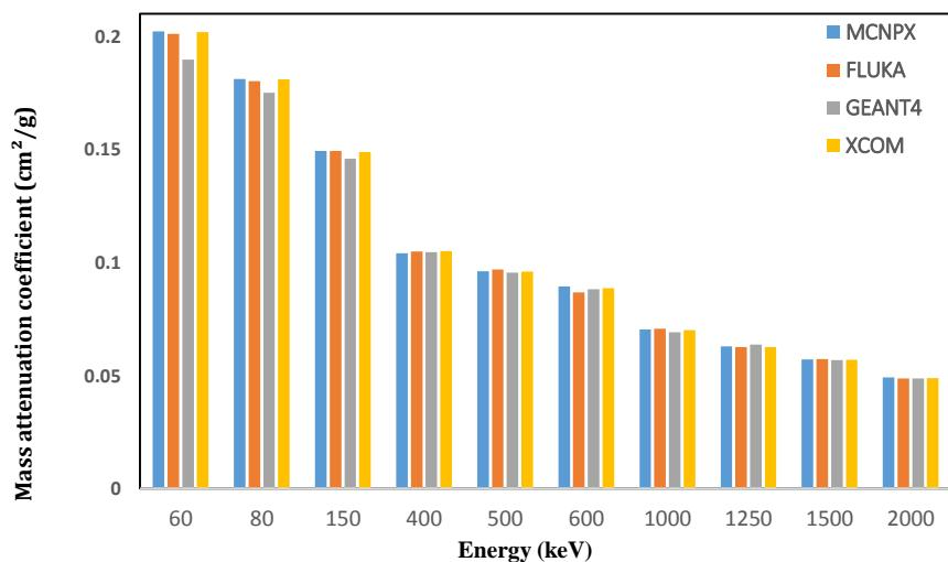
Figure 10. Mass attenuation coefficients for skin
