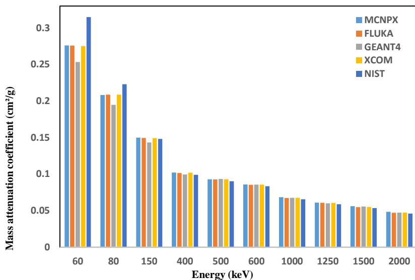
Figure 5. Mass attenuation coefficients for bone
