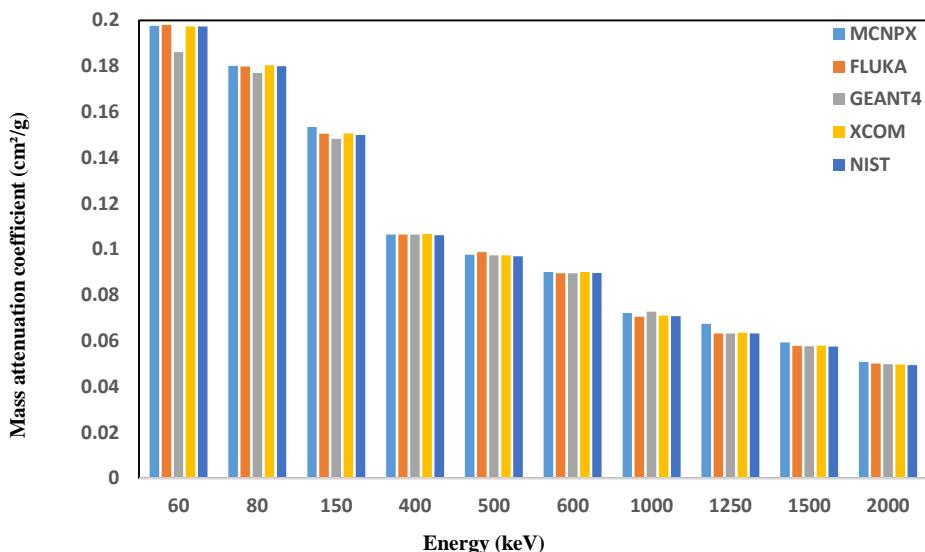
Figure 3. Mass attenuation coefficients for adipose tissue
