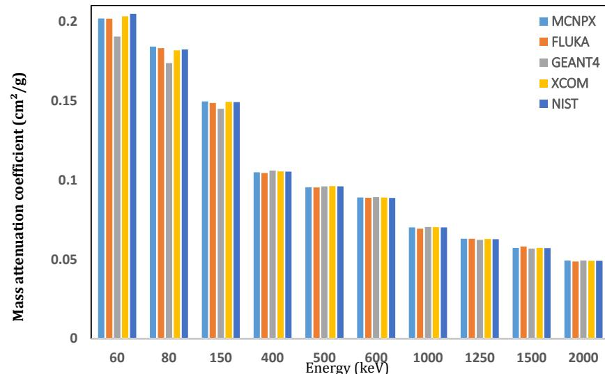
Figure 11. Mass attenuation coefficients for tissue
