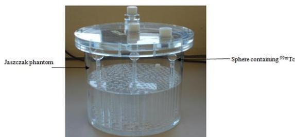
**Figure 1.** Lateral view of a Jaszczak Phantom filled with distilled water showing the position of the spheres filled with targeted activity concentration
