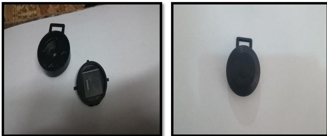
**Figure 2.** Detectors to measure radon
