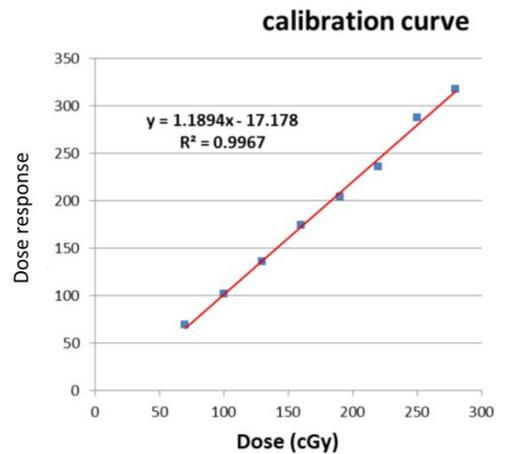
Figure 4. The calibration curve of thermoluminescent dosimeters
