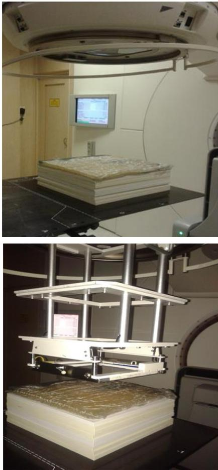
Figure 2. Left side, photon irradiation set-up; right side, electron irradiation set-up
