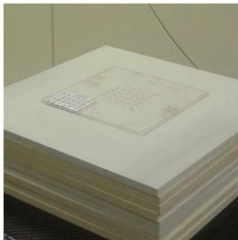
**Figure 1.** Thermoluminescent dosimeters container on 10 cm polymethylmethacrylate plates
