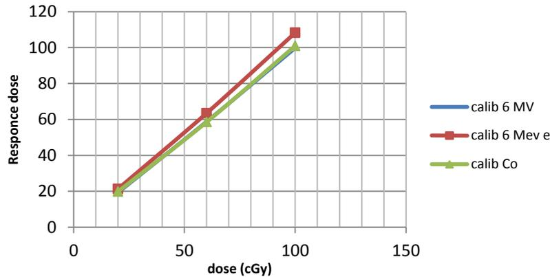
**Figure 7.** The dose response of thermoluminescent dosimeters (TLDs) calibrated in three groups, when irradiating with the <sup>60</sup>Co photon beam in different doses.
