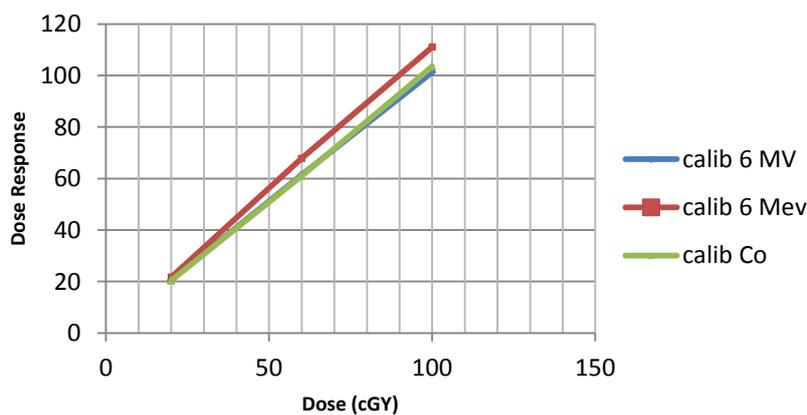
**Figure 5.** The dose response of thermoluminescent dosimeters calibrated in three groups, when irradiating with 6 MV photon in different doses
