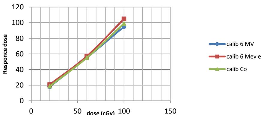
**Figure 6.** The dose response of thermoluminescent dosimeters calibrated in three groups when irradiating with 6 MeV electron in different doses
